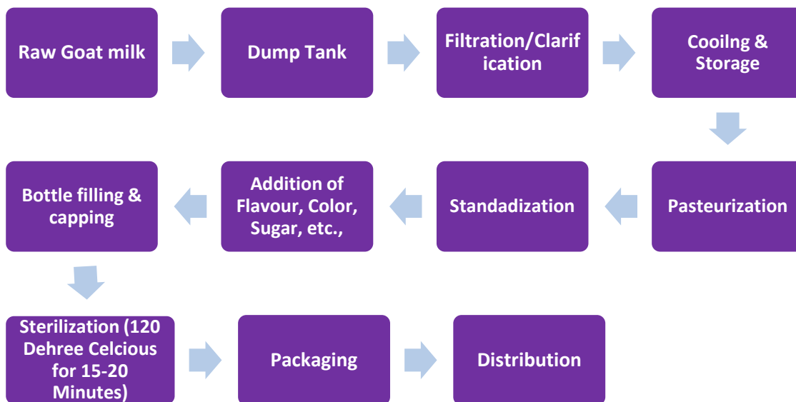
Figure 46: Steps for Goat Milk Sterilization
